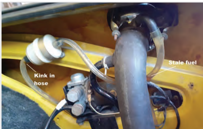
Pic 3: Kink in vent pipe, stale fuel and incorrectly mounted filter
